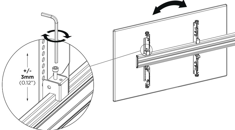
4. Micro-adjust depth of each display corner from wall
